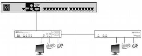
Tip: The local or remote console can be equipped with a KVM drawer instead of a set of keyboard, mouse and monitor. See the illustration below.
