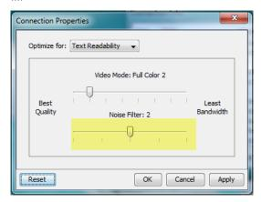
Moving the Noise Filter slider to the left lowers the filter threshold, resulting in higher dynamic video quality. However, more noise is likely to come through, resulting in higher bandwidth and lower frame rates.
