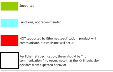
Note: For reliable network communication, configure the KX III and the LAN switch to the same LAN Interface Speed and Duplex. For example, configure the KX III and LAN Switch to Autodetect (recommended), or set both to a fixed speed/duplex such as 100MB/s/Full.
