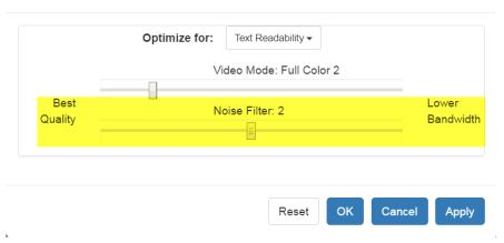
Moving the Noise Filter slider to the left lowers the filter threshold, resulting in higher dynamic video quality. However, more noise is likely to come through, resulting in higher bandwidth and lower frame rates.
