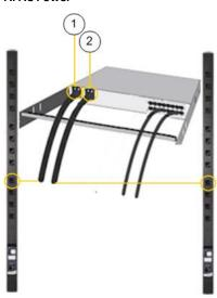
1. Use the power cords that came with KX III. Use both cords with AC power outlets for dual-power failover protection.
