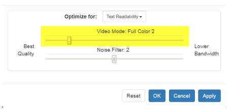
In general, moving the slider to the left results in higher quality at the cost of higher bandwidth and, in some cases, lower frame rate.
