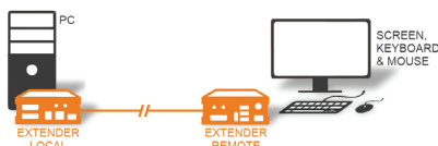
POINT TO POINT CONNECTION
