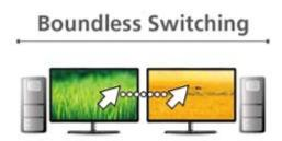
The mouse cursor can be moved **up**, **down**, **left**, **right**, or **diagonal** – off one screen and onto another to switch keyboard/mouse control to the adjacent computer. The audio and USB hub focus is also switched to the new computer.
