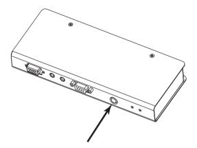
**Note:** Remote mode cannot be selected. The remote console can get control only when the Operating Mode Pushbutton on the CE350L / CE370L is toggled to *Auto* and the local console is idle. If the remote console is then idle for more than five seconds, the local console can gain access.
