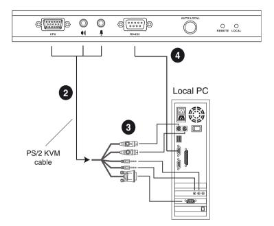
**Note:** The serial port on the CE350L / CE370L connects to the computer; the serial port on the CE350R / CE370RQ (not shown) connects to a serial device (optional).
