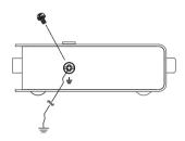
2. Make sure that the computer that the Local Unit connects to and the monitor that the Remote Unit connects to are properly grounded.
