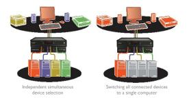
Examples of switching flexibility on the AV4PRO-DVI. Diagrams show the switching of connected devices across all connected computers and the selection of all connected devices to a single computer.
